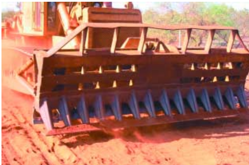
A 4 m stick rake with cutter bar front mounted on a large bulldozer is ideal for mesquite control. Photo: Jodi Graham
